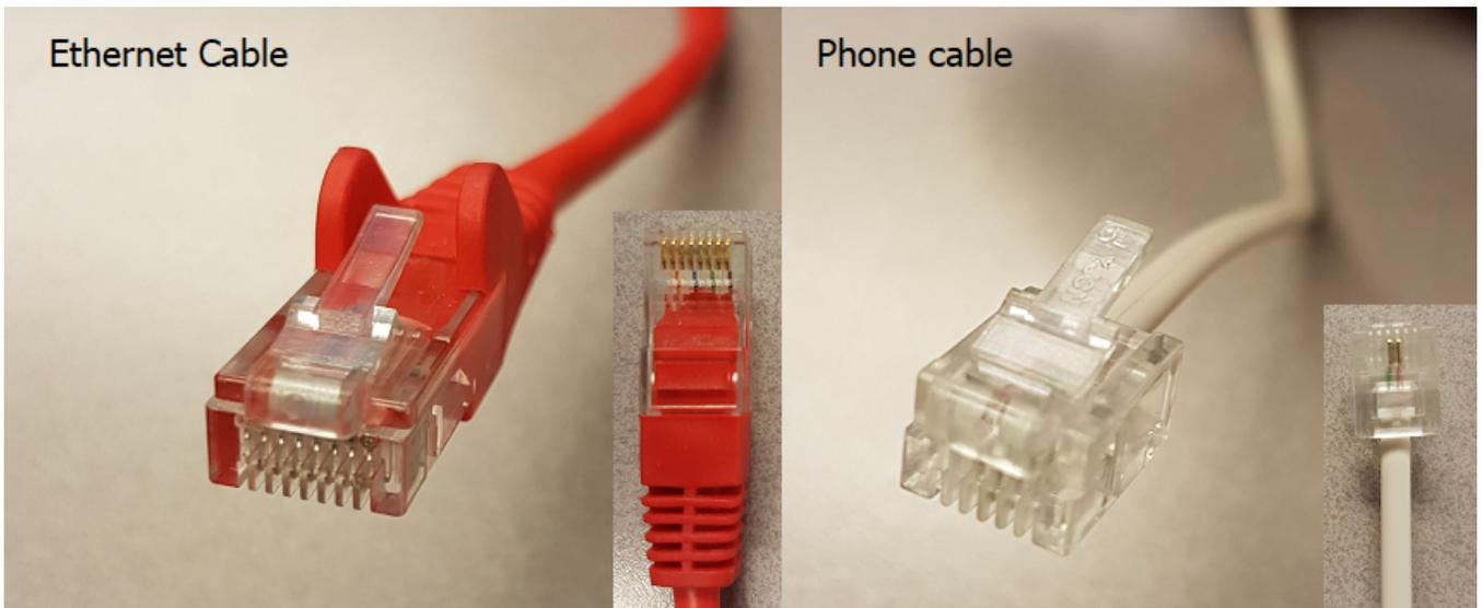
Important - ADSL telephone cables have very similar plugs to ethernet cables, but are not as
