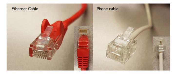
Important - ADSL telephone cables have very similar plugs to ethernet cables, but are not as
