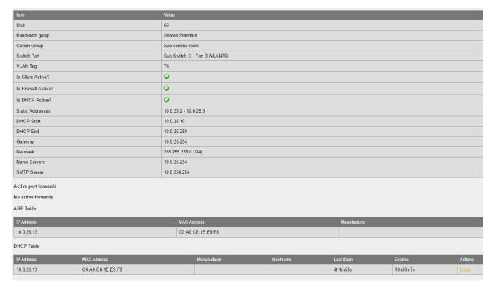
This shows a subnet address of 10.0.25.0, the available static address are .2 to .9; the address MESH will assign automatically go from .10 to .250.
